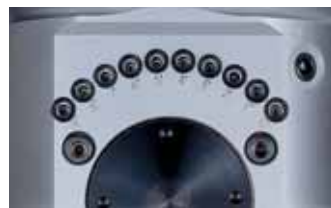
PRECISE ANGLE ADJUSTMENT Unique setting mechanism enables the spindle angle to be precisely set at 1° increments.
